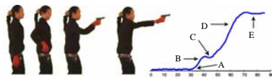
Figure 10. Stills from a video sequence; the right hand is tracked, and converted into a time series: A) Hand at rest; B) Hand moving above holster. C) Hand moving down to grasp gun. D) Hand moving to shoulder level, E) Aiming Gun.
