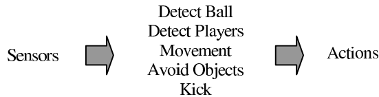
Figure 2: Brooks-style Layered Architecture for a Soccer Playing Agent.
