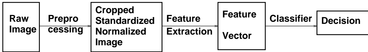
Figure 1: Architecture of a Typical Automated Visual Inspection System
