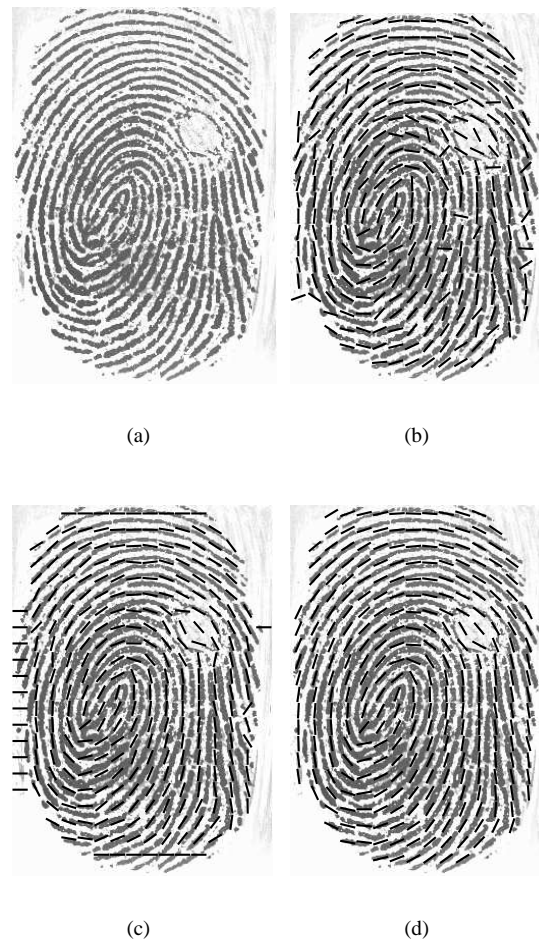
Figure 6. (a) A twin loop fingerprint image with a bubble blotch on top right; orientation fields estimated from: (b) the conventional gradient based algorithm; (c) the hierarchical scheme; (d) our weighted averaging method.
